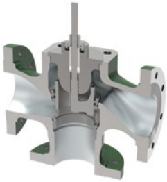
Figure 1.8 Three-Way Globe Valve
