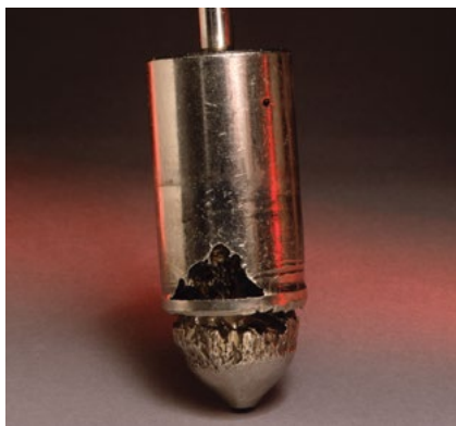
Figure 5.8 Typical Appearance of Flashing Damage
