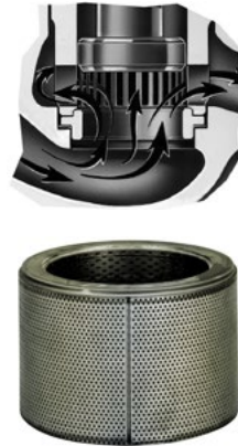
Figure 5.10 Valve Trim Design for Reducing Aerodynamic Noise
