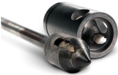
Figure 5.9 Typical Appearance of Cavitation Damage
