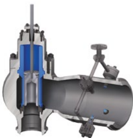
Figure 7.10 Cross-Section View of Steam Conditioning Valve
