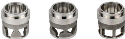
Figure 1.7 Cages (left to right): Linear, Equal-Percentage, Quick-Opening
