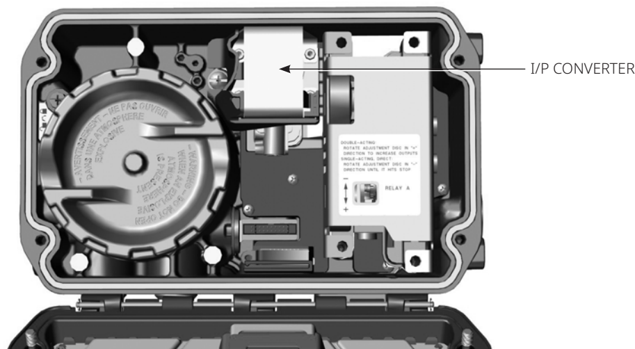
Figure 12. I/P Converter Location
