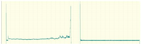
The graph above represents motor power trace. You can see as the valve is closing, the graph has multiple spikes throughout the stroke. The open side is smooth (as expected). This is an indication of upper drive sleeve bearing wear or damage.
