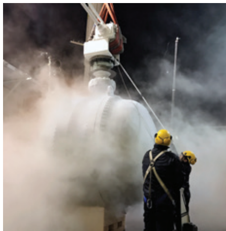
A Vanessa 96" double flanged cryogenic valve tested at Lugagnano plant (Italy).
