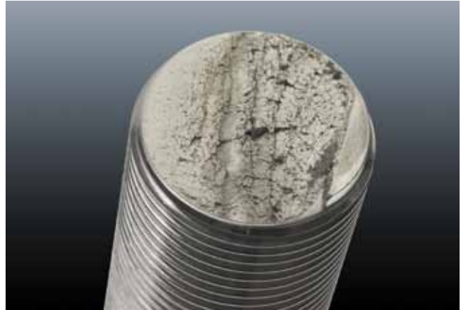
Control valve stem/shaft breakage is a common fatigue failure due to heavy vibrations within the system.
